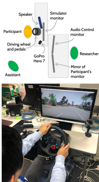
Figure 3: The Wizard-of-Oz setup. [Top] The overhead view of the room with the location of participant, researcher and assistant. The researcher sees a mirror of the participant's monitor. Every time the driver comes near a decision point, the researcher plays the recorded instructions and conversations. [Bottom] A participant using the setup. In front are: 1 monitor for driving simulator, 1 GoPro camera for capturing utterances while thinking aloud, 1 steering wheel set, and 1 speaker.
