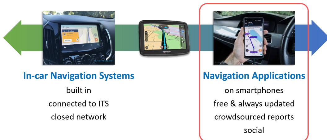
Figure 1.1: The spectrum of navigation tools that are available commercially for drivers. Leftmost are in-car navigation systems which typically come with a vehicle. Such navigation tools are different per car make and model. One of their main advantages is that they can communicate with other cars of the same car make and access to maps do not need connection to the Internet. In the middle are satellite navigation tools or GPS devices. These can be bought separately from navigation companies (e.g. Tomtom and Garmin) and can be mounted on any car. Rightmost are modern navigation applications like Google Maps and Waze. They are run on smartphones and access to the most recent maps and route information is mostly free.
