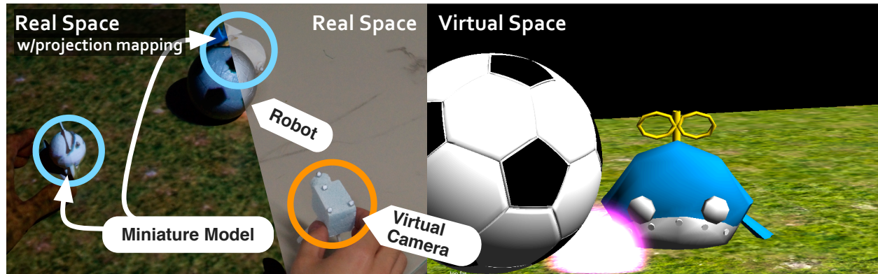
Figure 1: Left: Miniature models including a camera and a robot enhanced by AR technique. Right: A view from the virtual camera.
